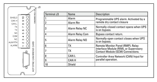
Figure 22 XSlot Hot Sync card and terminal interface
